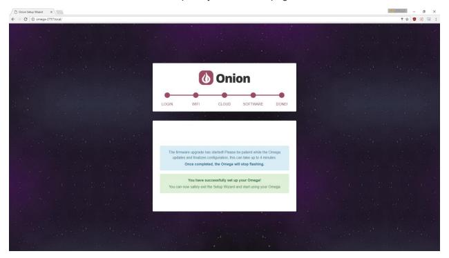
At the end of the installation process, the Omega will automatically reboot. It will be ready for use when the Omega's LED stops flashing and remains solid.
