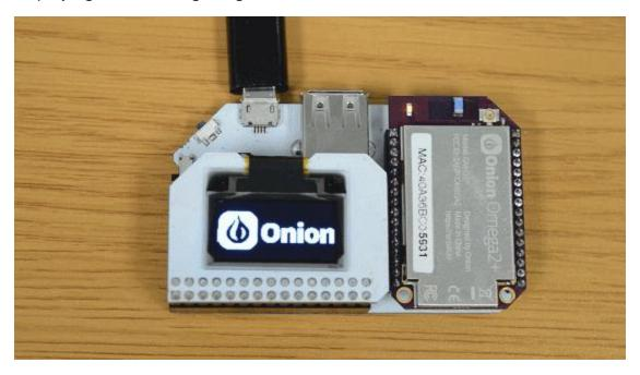
This Expansion communicates with the Omega using the I2C protocol, it's I2C device address is 0x3c. If you're curious, check out the article on I2C.
