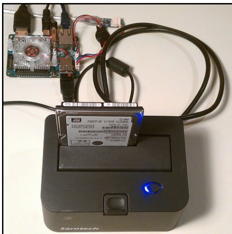
Docking system with SATA HDD storage device attached to XU4
