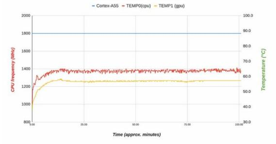
Even when assembled in the case, the CPU temperature did not exceed 75°C and thermal throttling did not occur.
