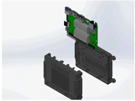
The SOC in the M1S is the RK3566, which is the younger sister of the RK3568 used in the original M1. This allows most of the software development to be reuse d. Because the bootloader and kernel settings are different, existing OS images for M1 cannot be used as-is, but porting is quickly possible through a simple proces s.
