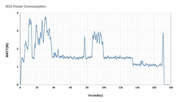
When performing a CPU stress test without either HDMI output or Ethernet connection, the power consumption is about 3.2 Watts. This shows an energy savings of about 25% compared to the 4.3 Watts of the original ODROID-M1 under the same test conditions. Note that the computing power of ODROID-M1S has been m easured to be 5-10% lower than that of M1.
