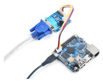
or you can use a USB to serial board and power on the whole system at the MicroUSB port with a 5V/2A power:
