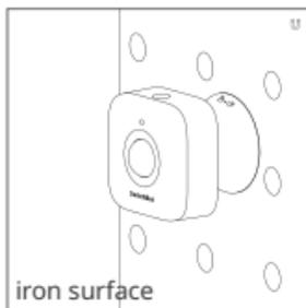
You can also stick the Base to a flat surface using the 3M Sticker. After Motion Sensor is properly installed, tilt it to a desired angle.
