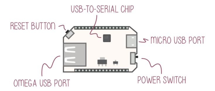
The Mini Dock allows for easy communication via the USB-to-Serial chip located in the center of the board.
