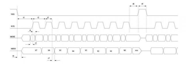
• The SPI bus writing a command to the LoRa chip will trigger the switching of the internal state machine mode. It should be noted that the low level of the BUSY pin indicates that the internal idle is allowed to receive commands, and the high level indicates that the internal occupied cannot accept the SPI command. The SPI bus needs to wait for the BUSY pin Pull low again to continue reading and writing operations, TswMode is up to 3.5ms.
