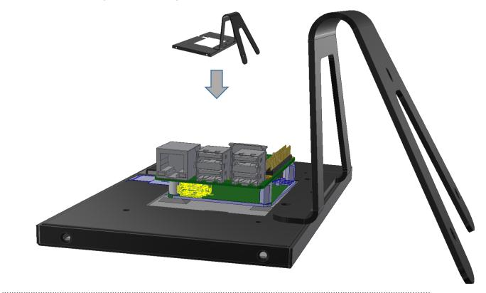
4. Mount the back plate with the M3 pan head screws. Add the self-adhesive rubber feet
