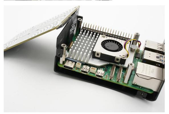
b)The Pimoroni NVME will be assembled upside down like the below image. Secure the HAT with the 4 pan head screws.
