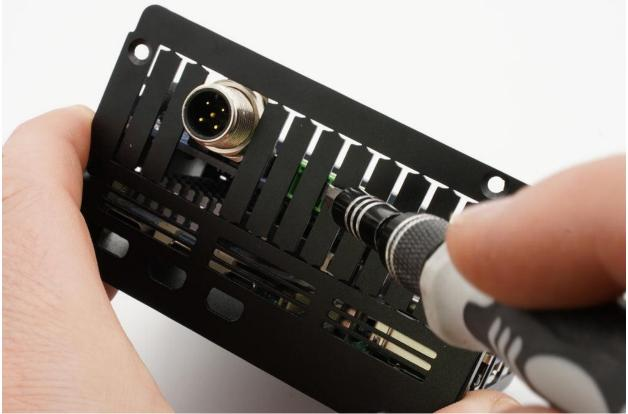
5. Put together the side panels with the bottom piece and then Put together the top part.
