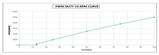
(The fan will be able to start when the duty cycle is 13%)
