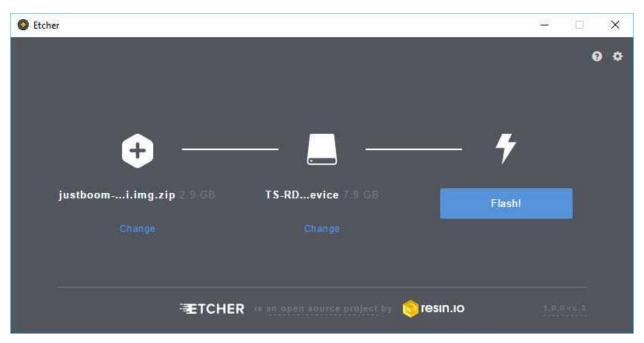
**Step 2** – Use our favourite tool <u>Etcher</u> to transfer the image onto a Micro SD card. Select the image you want to flash, choose the drive on which to write and flash the card.
