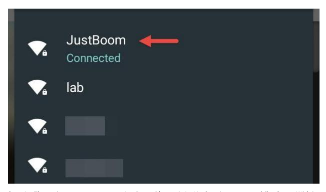
**Step 1** – The easiest way to connect to JustBoom Player via its HotSpot is to use a mobile phone. With it connect to the JustBoom SSID using password **justboom**.
