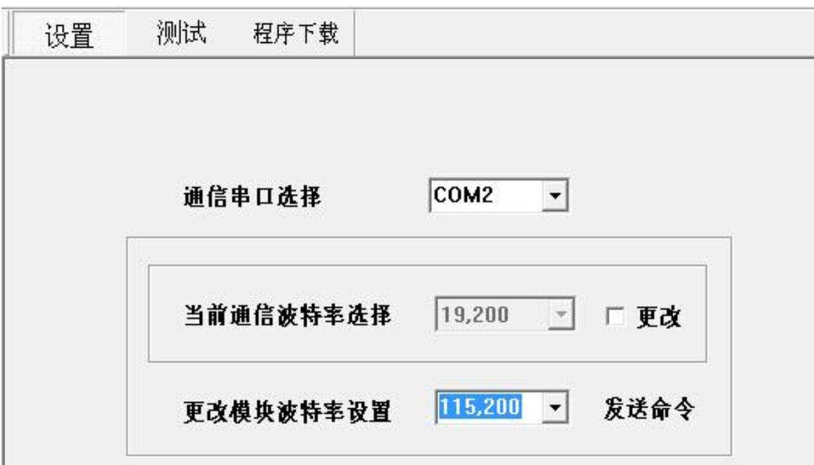
Notice: When the baud rate of the module has been modified to 11520, the baud rate of your PC should be set to 115200 as well. Otherwise, it may cause communication failure.
