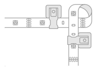
Please do not fold or twist the LED Strip Light as shown in the picture below. Bending the LED Strip Light will cause excessive stress on the bent areas (such as circuit boards, resistors, LED chips, etc.) and may lead to malfunction.
