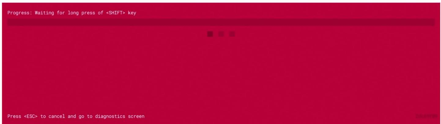
In the background the Raspberry Pi is still looking for a bootable image, but you can now start a network installation by holding down the SHIFT key. You will then be prompted to connect your Raspberry Pi to the network with an Ethernet Cable.
