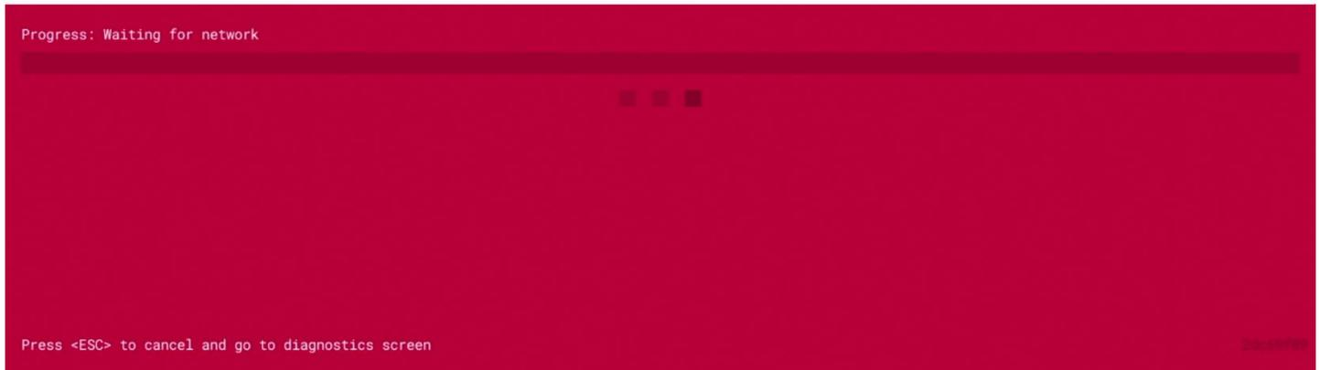
Plug your Raspberry Pi into the network using an Ethernet cable. When it detects a cable has been inserted it should start downloading the Raspberry Pi installer. If the download fails, you can repeat the process to try again.
