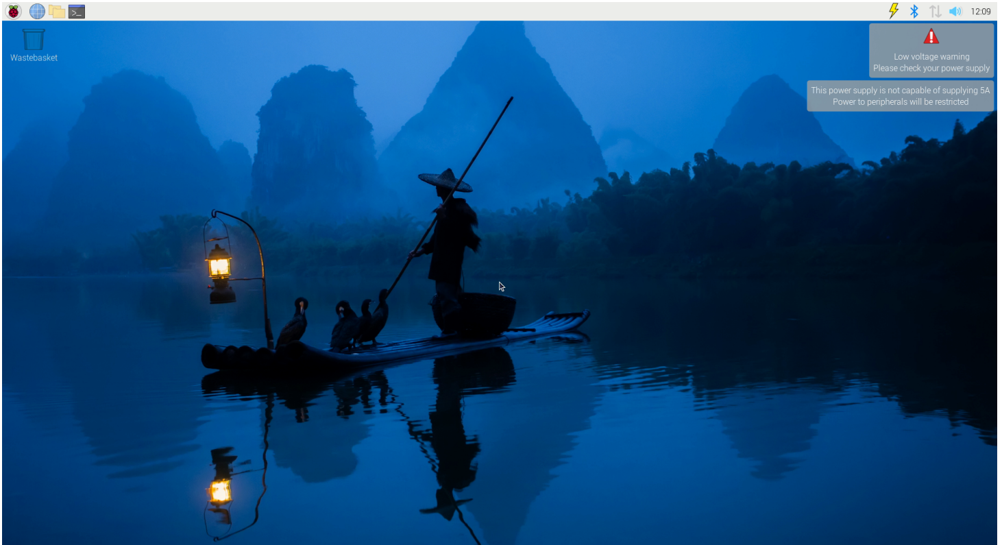
On-screen warning of under-voltage event
