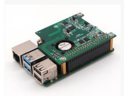
ROCK Pi 23W PoE HAT is a HAT accessory designed for Raspberry Pi, ROCK Pi 4, and Jetson Nano. The 23W PoE HAT allows you to power your Raspberry Pi, ROCK Pi 4 or Jetson Nano using Power over Ethernet—enabled networks; for this product to be used, the network it is connected to needs to have power-sourcing equipment installed.
