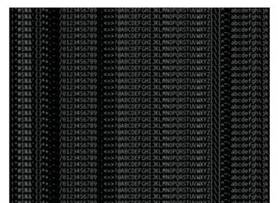
Shows off chained DMA to generate scanlines out of glyph fragments via DMA/PIO
