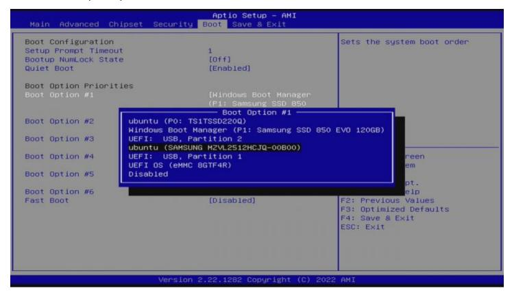
• Instead of entering the BIOS menu to select a boot device, the "F7" key can be used at power on or reboot. This will present a menu with the list of connected storage devices and you can select one of them to boot from.
