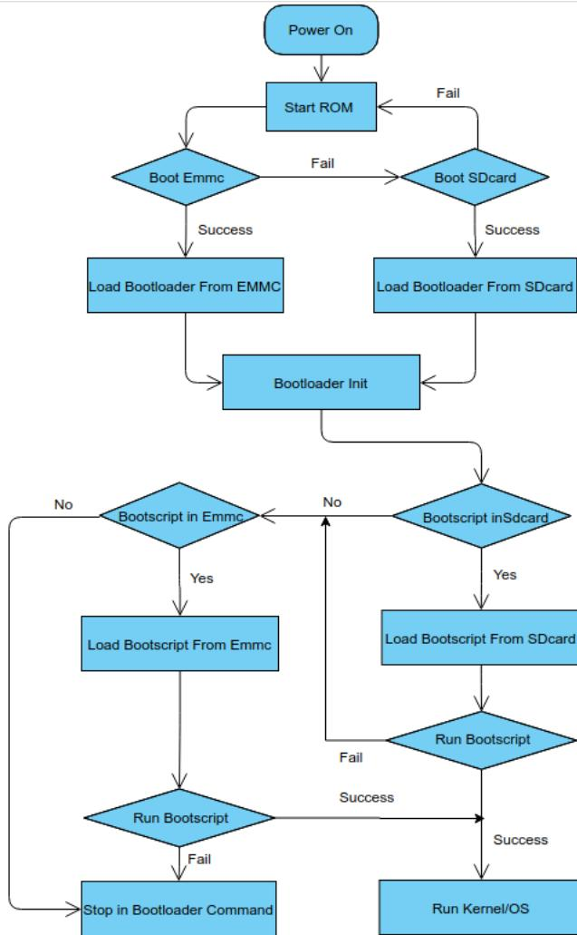
Check bootloader loaded from SDcard or EMMC at the beginning of the console debug messages
