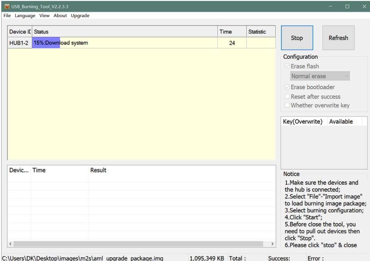
4. After Burning successfull, Unplug the type-c usb and connect to power supply adaptor to startup.
