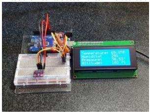
The program below implements a simple weather station using the GY-BME280 module and a LCD2004 20  $\times$  4 LCD to display the info.
