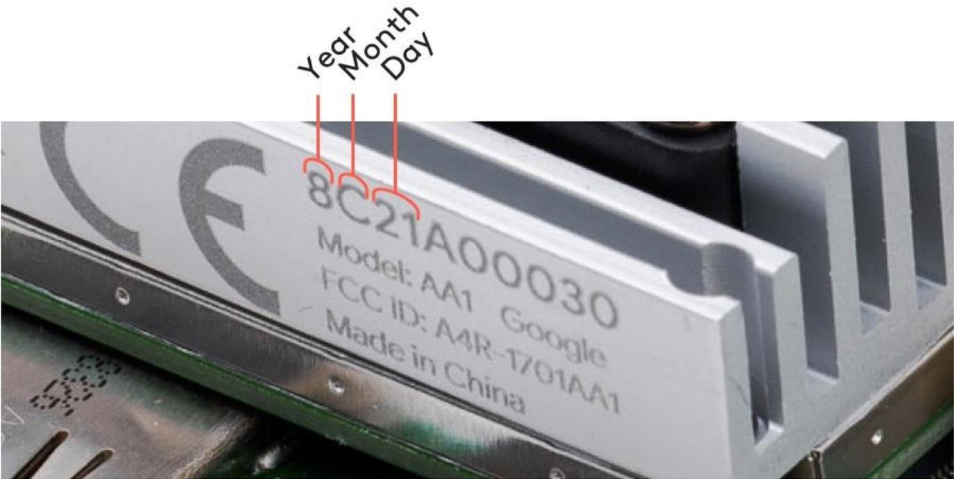
**Figure 8.** The manufactured date in the serial number
