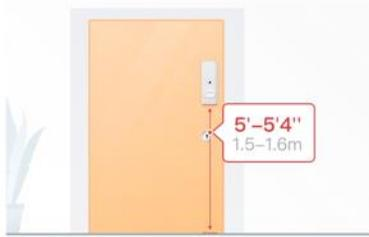
Peel & Lightly place on a closed door
