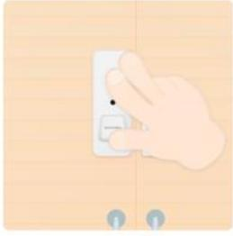
Using the sticker lets you start with a light touch so you can adjust the placement. Then you can make it more permanent with pressure. Make sure the installation area is clean and dust free.
