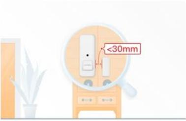
Align the open-close magnet with the bottom of Contact Sensor. Make sure the max distance between Contact Sensor and the magnet is under 1.2 in (30 mm), the light would glow white when they are close together.
