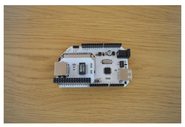
NOTE: The Ethernet Expansion does not plug in ALL THE WAY like the Omega does. The pin will be exposed at the top (refer to image above)
