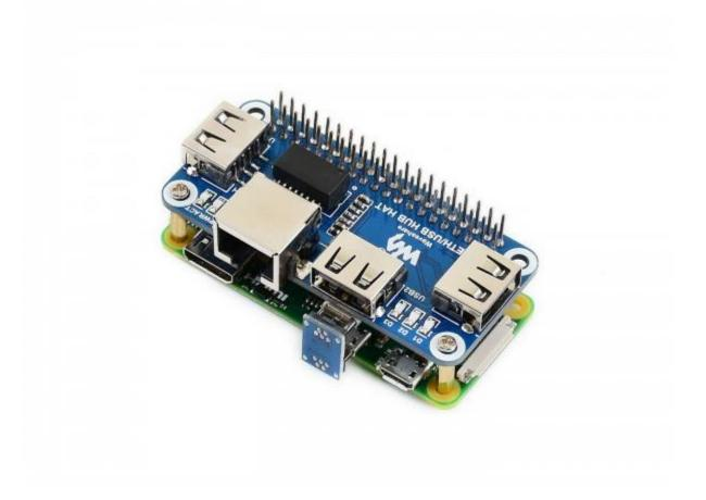
• Connect Network cable to RJ45 interface of ETH/USB HUB HAT.
