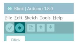
After the compilation and upload process, you should see the message *Done Uploading* and the built-in LED of the board should start blinking.
