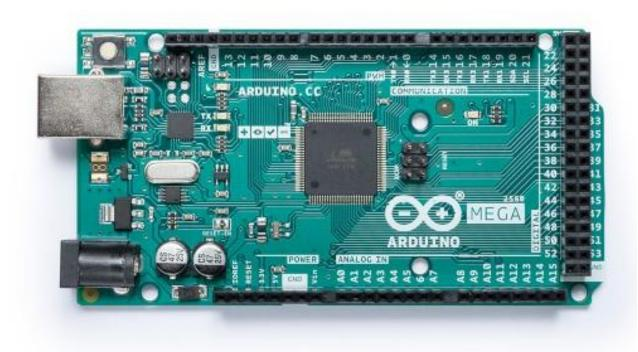
Arduino Mega 2560 is designed for projects that require more I/O lines, more sketch memory and more RAM. With 54 digital I/O pins, 16 analog inputs and a larger space for your sketch it is the recommended board for 3D printers and robotics projects. This gives your projects plenty of room and opportunities maintaining the simplicity and effectiveness of the Arduino platform. This document explains how to connect your Mega2560 board to the computer and upload your first sketch.
