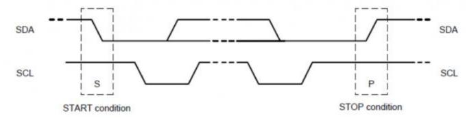
START signal: When SCL is high level, SDA jumps from high to low to start transmitting data.
