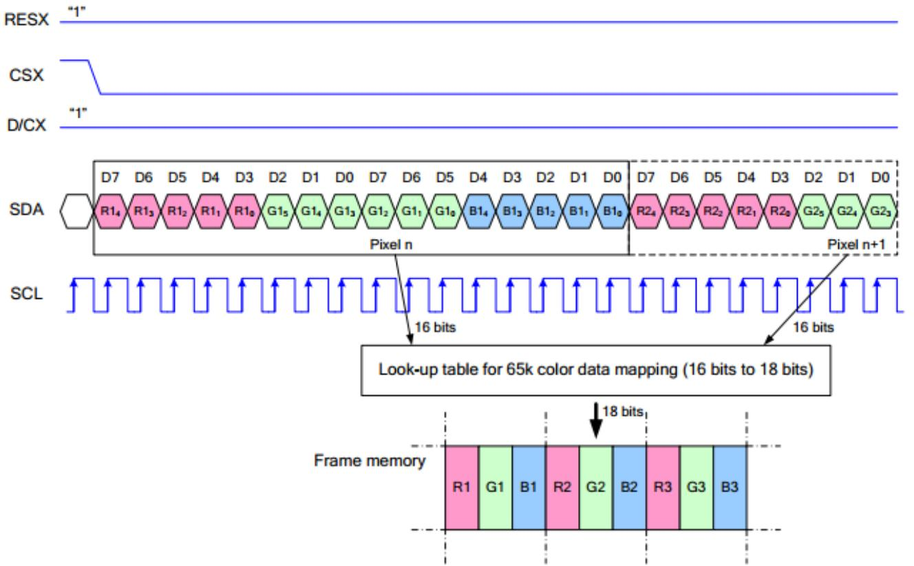
Note: It is not like the traditional SPI protocol, it only uses MOSI to send data from master to slave for LCD display. For details please refer to Datasheet Page 105.
