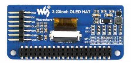
The interface of 2.23inch OLED HAT is default SPI interface, that is 0R resistors are soldered to SPI sides. If you want to use I2C interface, you need to solder the 0R resistors to I2C side,
