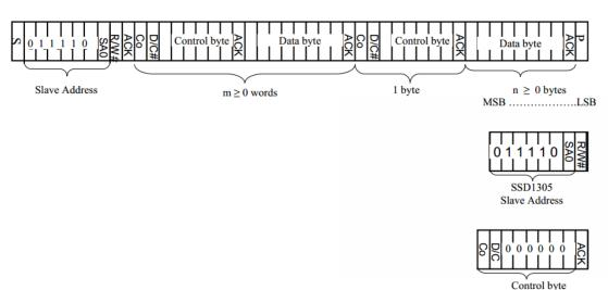
At the begging, the Master device sends a byte (7 bits address and 1 bit R/W)to slaver device and wait for a response.
