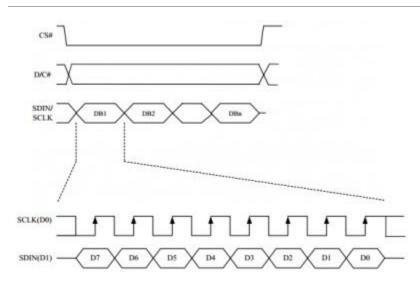
Note: Different from the traditional SPI protocol, the data line from the slave to the master is hidden since the device only has display requirement.
