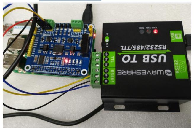
Connect <u>USB TO RS232/485/TTL</u> to the computer, open the serial port assistant software, select the corresponding serial port, and set the baud rate to 115200.
