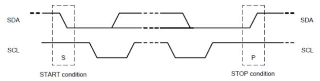
Start signal: When SCL is high level, SDA jumps from high level to low level, and starts to transmit data.
