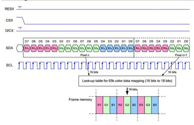
Note: Different from the traditional SPI protocol, the data line from the slave to the master is hidden since the device only has display requirement.
