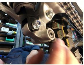
22. Fit new M10 bolt and single washer from left into the bottom of the shock fork, whilst aligning it the knuckle joint. Sometimes it is required to rotate the fork slightly to get the alignment correct. This can be done using a small bar or long allen key through the bushes of the shock fork.
