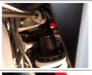
19. Place washer onto a long allen key or screw driver, then place the tip on the threaded end of the bolt, use another small tool to push the washer onto the bolt. Alternatively use a small telescopic magnet to secure the washer to the thread.
