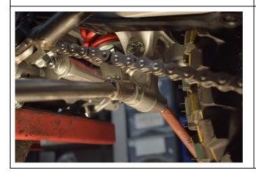
2. Using 17mm socket from left side, and 14mm spanner on head of bolt on right, undo the nut and remove the long bolt holding the dog bone link to the knuckle joint.
