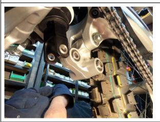
21. Replace knuckle joint into the swinging arm, using the largest bolt from the left. Then place large washer onto bolt and replace large nut. Tighten slightly.
