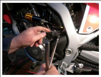
13. Replace the plastic sprocket guard, fit lower screw then upper screw with black metal sensor cover, tighten loosely.
