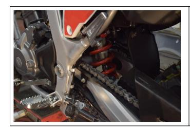
7. Remove top bolt and lower shock out and under the swinging arm.
