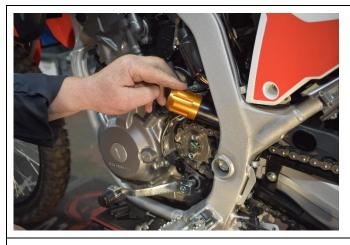
11. Feed the adjuster handle and mounting bracket through the space above the gearbox sprocket, and into the mounting position. At the same time lift and support the rear shock up into the bike.
