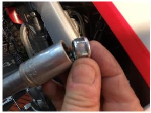
20. Use a 17mm socket to replace the nut on the top bolt, and tighten slightly.
