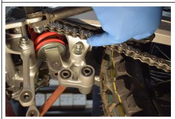
5. Using 17mm socket from left side, and 17mm spanner from the right undo the nut and remove washer. Then remove knuckle joint bolt and remove the knuckle joint from swinging arm.
