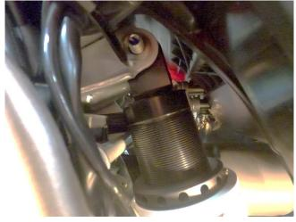
12. Once the adjuster handle is through, push the shock up and insert the top shock bolt from the right, with a small amount of grease applied.
