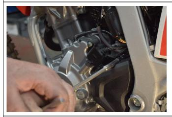
8. Remove both sprocket cover screws with 8mm socket, and the screw holding the black metal sensor cover to engine.
