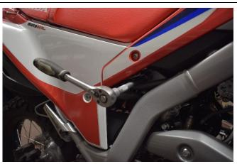
6. For CRF300L & RALLY: Using 17mm socket from left side, and 14mm spanner on right undo the nut and remove washer.
