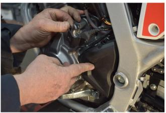
9. Remove the screw to the left of the sensor cover, and discard.
