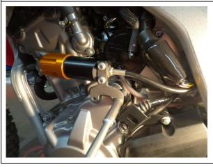
14. Fit handle adjuster to engine casing and insert rear adjuster bracket screw on top sensor cover with original screw.
