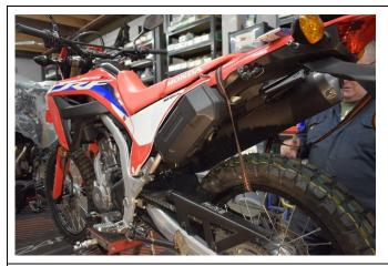
3. Lift the rear wheel up so that the swinging arm is horizontal, and secure with a strap or a block under the wheel. This will aid in removing and replacing the shock later.
