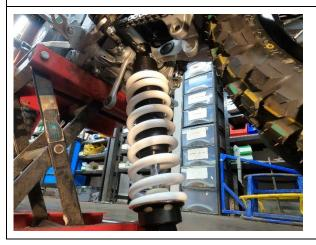
10. Insert new shock with HPA fitted into the swinging arm area of the bike, ensuring the flat face on the top preload nut is facing towards the front of the bike.
