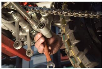
4. Using 17mm socket from the left side, and 14mm spanner on the right, undo the nut and remove the lower shock bolt, discard both bolt and nut.
