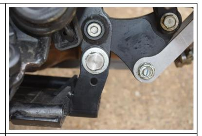
11. Carefully lift the front of the engine to meet billet mounts, apply Loctite and secure using M10 X 25 bolt and M10 washer provided.
