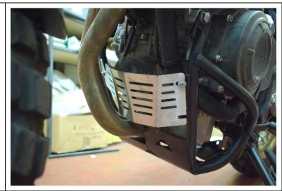
18. Insert both M6 x 15 screws on the left side to locate into Front Cover, use washers & nylon nuts on inside, fully tighten all 3 screws.
