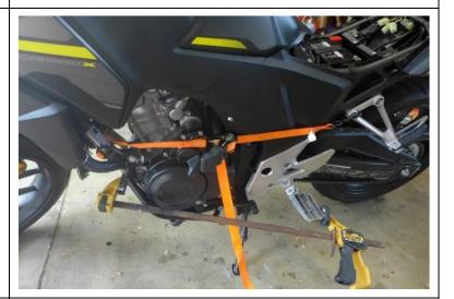
9. Lay engine guard under the bike and lift the rear bracket to meet the pivot pin mount as shown.
