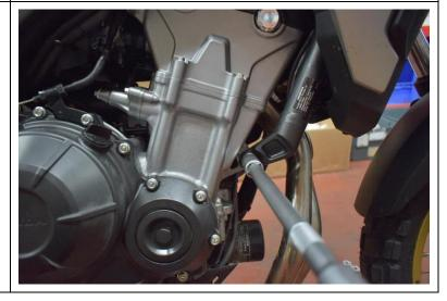
6. Apply Loctite and re-insert OEM engine mount bolt through frame and billet mount, taking care not to cross thread the bolt.
