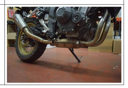
3. Remove rubbers and bushings from plastic guard and fit to stainless guard provided.
