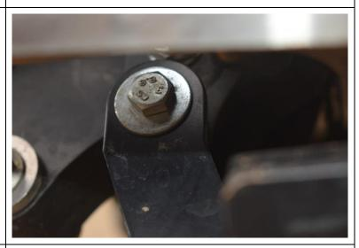
16. Fit M6 x 15 screw into r/hand lug on front of Engine Guard, with washer and nyloc on inside, leave undone.
