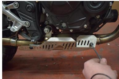
5. Using 14mm socket, carefully remove engine mount bolt from one side of the bike only. Remove the OEM aluminium washer and replace with billet engine guard mount pointing downwards.
