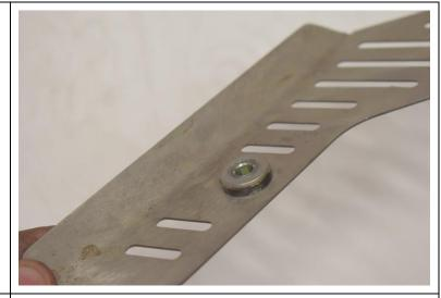
Using OEM bolts, refit the stainless guard to the catalytic converter using low strength Loctite.
