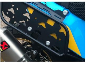
7. Tighten both upper M8 CSK screws (18Nm) and both lower M8 CHS (18Nm) with 5mm and 6 mm allen bits respectively.
