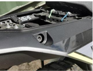
2. Before fitting the racks, ensure the rubber buffers are attached as per photo.
