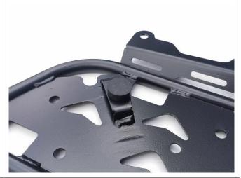
3. Use a small amount of Loctite on M8 x 70 CSK screws and attach right panel, using long tapered spacers as shown.
