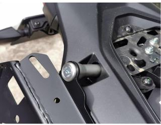
4. Remove both M8 screws attaching the footrest hangers.
