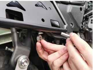
6. Remove M8 silencer bolt, washer and nut, then insert M8 x 35 CSK screw with form washer from outside of rack through front lower hole. Place the thick spacer, silencer support bracket, then lower rack support L bracket, fit M8 washer and nyloc nut, do not tighten.
