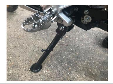
14. Check stand returns under spring pressure, and then check switch works by trying to start engine with 1st gear engaged and side stand down, it should not start, but be careful, and be ready to pull clutch lever in in case the engine starts!!!
