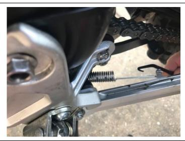
2. Using 14mm spanner, undo and remove nut on stand pivot bolt, as shown.
