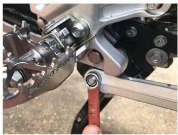
3. Using 10mm hex Allen key (if no centre stand fitted) or 10mm hex bit and 10mm ratchet ring spanner (if centre stand fitted) to undo and remove rear pivot bracket bolt.
