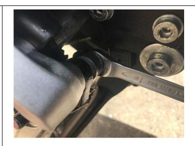
4. Repeat above with front pivot bracket bolt, remove bolt and metal switch cover from assembly.
