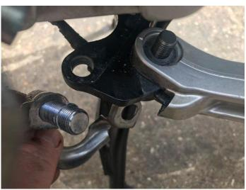
5. Turn over stand and bracket, then remove M6 switch bolt, using 10mm spanner.
