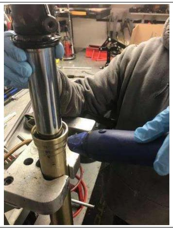
3. Using a sliding action, remove inner fork stanchion from outer leg by repeatedly sliding backwards and forwards until it comes out completely.
