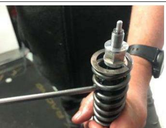
5. Each preload cap for the fork comes complete with three plastic washers, these can be mixed in any combination as long as they have the same thickness for each fork cap.
