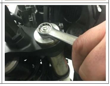
8. Slacken both bolts on the lower right-hand triple clamp, with 10mm spanner, and slide out complete fork leg.
