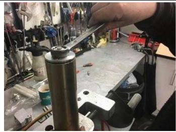
4. Slide up the fork lower to expose the fork spring, pull down the fork spring slightly, and hold the locknut under the cap with a 17 mm spanner, then twist off the cap completely with 19mm spanner.
