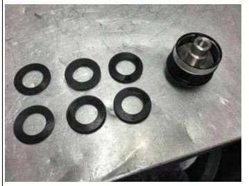
6. Place the required plastic washers onto the top of the spring, and then screw on the fork cap by hand until resistance is felt. Tighten fully using a 22 mm spanner on the fork cap and a 17 mm spanner on the aluminium nut.
