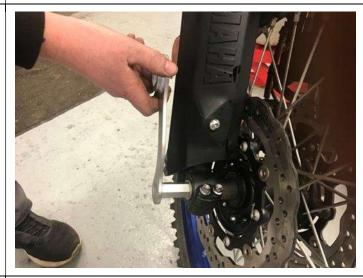
5. Tighten axle fully by hand.
