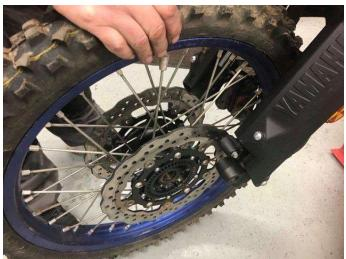
5. Using 5mm Allen key, remove both screws on the lower front and side of fork leg.
