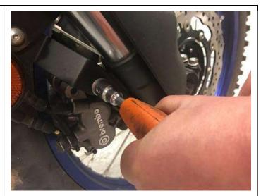
7. Remove bike from stand and pump front brake gently until the pads bite, then holding the front brake on, pump the forks up and down before tightening both pinch bolts on lower right fork leg with 10mm socket.
