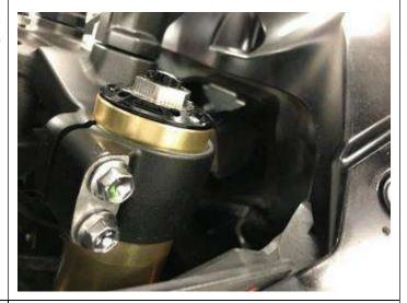
2. Fully tighten the fork cap, using the special pin spanner, to hand tight. Tighten both upper and lower fork pinch bolts with a torque wrench to the recommended settings listed below.
