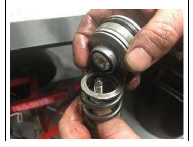
5. Remove the fork spring and invert the fork leg to drain the oil from the leg, try and put one finger over the top of the piston rod to prevent the 5 mm diameter aluminium rebound needle from falling out when the fork leg is upside down. It is useful to stroke the piston rod up and down slowly to help remove the oil from inside the fork leg.
