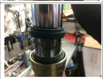
11. Lastly, push in the dust seal, and wipe any excess oil from the whole assembly.
