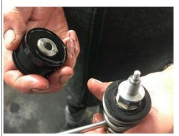
Pour in 100ml of 15W good quality fully synthetic fork oil. Replace fork cap only on to piston rod by hand then pull up outer tube and screw fork cap in by hand using tool provided.
