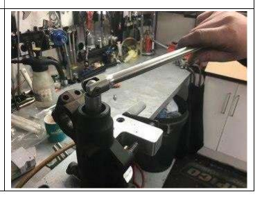
3. Invert the fork leg again and clamp in a suitable vice and using a 19 mm spanner undo fork cap completely.
