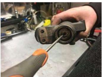
2. Invert the fork leg and hold in a suitable clamp then using a 14 mm hexagon bit, undo the compression adjuster at about half a turn to break the seal.
