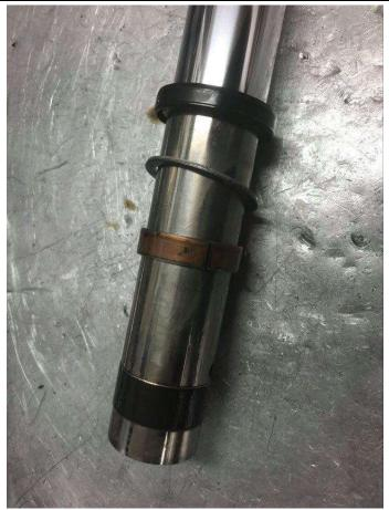
4. Prize off the top bush by opening the gap and sliding it off the top of the fork leg, the next bush slides straight off, along with the steel washer, then the oil seal, metal clip and dust cover.
