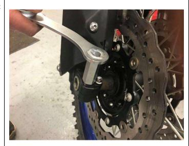
4. Using our special tool, or a 19 mm hexagon bit, undo front wheel spindle and remove from axle whilst supporting the front wheel.
