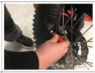
6. Undo slightly, both top pinch bolts on top triple clamp, a couple of turns using 10mm spanner.
