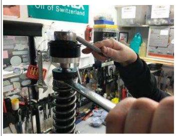
7. Check that the whole assembly looks correct, and in line, slide the fork outer up to meet the fork cap, start tightening by hand, until resistance can be felt, then use the special pin tool provided, to tighten the cap into the tube as tight as possible by hand.
