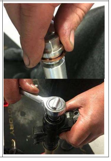
2. Using 22mm and 17mm spanners, pull down fork spring and remove the fork cap and fork spring (along with any plastic washers).
