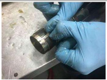
5. Clean the chrome leg completely to remove any debris and then rebuild in the opposite order. To prevent any damage to the fork seal from the sharp edge on the top of the chrome tube, it is best to use a small piece of plastic bag or a professional plastic fork tube cap over the open end of the leg, lubricate the plastic and the fork leg with new fork oil to aid insertion of the new parts.
