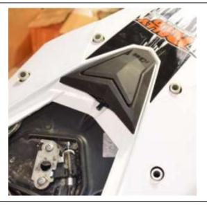
NOTE : DO NOT USE LOCTITE OR SIMILAR ON THESE BOLTS, THEY ARE PRONE TO BECOMING STIFF AND WILL DAMAGE THE THREADED INSERTS.
