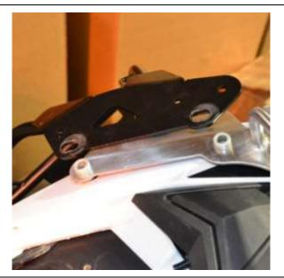
USING LONGER M8X70 BOLTS AND FORM WASHERS LOCATE THE THREADED INSERT AND TIGHTEN ALL FIXINGS LOOSELY, BEFORE FULL TIGHTENING ALL.
