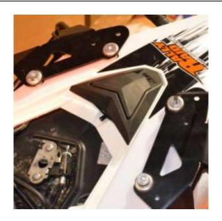
BE SURE THE SPACERS ARE SITTING CORRECTLY AS SHOWN AND THE FRAMES ARE NOT TOUCHING OR OBSTRUCTING ANY BODYWORK.
