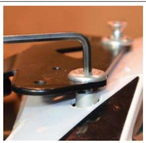
NOW ATTACH THE LOWER FRAME MOUNTS TO THE BIKE USING THE M8X30 SCREWS (APPLY LOCTITE) AND 19MM SPACERS PROVIDED, DO NOT OVERTIGHTEN.
