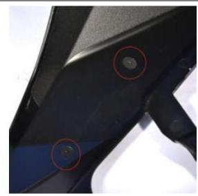
INSERT 4 X 22MM SPACERS INTO THE DRILLED HOLES, SO THEY SIT ONTOP OF THE THREADED INSERTS.
