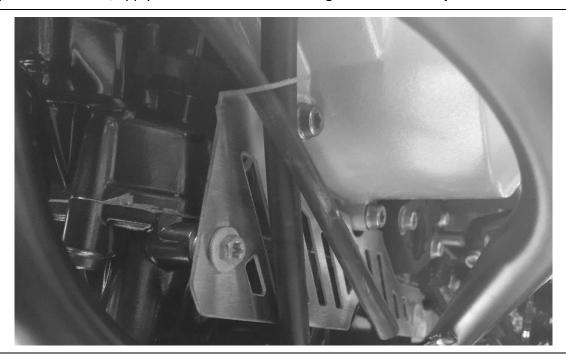
11. Insert rubber breather tubes into the hole in the folded tab on the left side plate.
