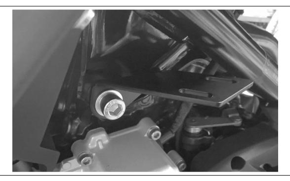
6. The brackets are handed, and the tabs should point backwards, as per photo. **Do not tighten the screws fully**, leave them so the brackets can rotate.
