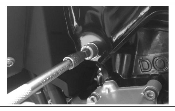
4. Undo both upper engine mounting M10 Allen screws and washers, do not discard them.
