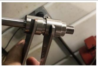
8. Slide in the new fork spring, ensuring that the smaller tapered end of the fork spring is at the top. Slide on the larger aluminium spacer over the spring and down to the gold fork tube.
