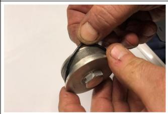
5. Screw on 25mm extension piece to damper rod until the thread on the damper rod bottoms out inside the extension piece.
