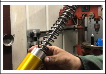
9. Slide on the smaller aluminium sleeve over the extension piece and then screw on the new pre load cap to the extension piece. Using 16mm spanner on the new nut and 22mm spanner on the centre of the pre-load cap, lock the two together.
