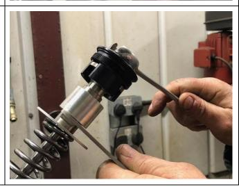
10.Pull down the spring to release the pressure and remove the C washer, then let the spring and the small sleeve go back up to seat on the underside of the preload.
