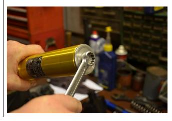
3. Whilst holding fork cap with 17mm spanner undo the 16 mm locknut underneath on damper rod and remove fork cap, screw locknut back down to bottom of thread by hand.
