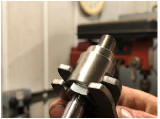
6. Tighten down new fork cap on to extension piece by hand until the two faces meet.
