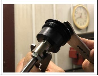
8. Fit the original O ring onto the new preload cap and screw the new preload cap into the outer tube by hand, apply grease to the O ring before assembly.
