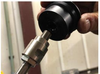
7. Holding the new fork cap with pin spanner provided and the extension piece with the 16 mm spanner provided and lock the two together.
