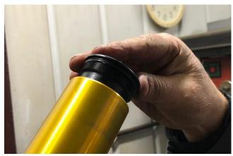
Replace the fork leg back into the triple clamp with approximately 10 mm of gold fork tube protruding through the top triple clamp, tighten both lower pinch bolts in bottom triple and then fully tighten the fork cap with the pin spanner provided.
