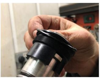
11. Fit the old O ring onto the new preload cap and screw the new preload cap into the outer tube by hand, apply a bit of grease to the O ring before assembly. Hold the gold outer tube by hand and tighten gently the preload cap using the pin spanner provided.
