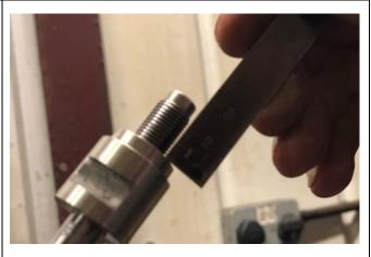
7. Screw on 25mm extension piece to damper rod until the thread on the damper rod bottoms out inside the extension piece. There should be a few mm gap between the underside of the extension piece and the top of the new nut.
