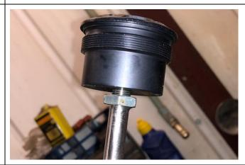
6. Holding the new fork cap with pin spanner provided, wind up the original oem nut on the damper rod with the 16 mm spanner provided and lock the two together.
