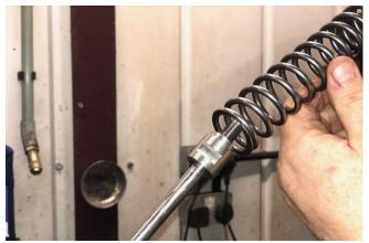
7. Pull down the fork spring using two hands and with the help of another person slide the C washer supplied with the kit between the top of the fork spring and the underneath of the new nut to hold it in position then you can release the spring safely.
