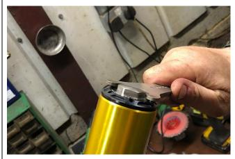
12. Remove from vice and pump fork leg up and down by hand to check for free travel. Replace the fork leg back into the triple clamp with approximately 10 mm of gold fork tube protruding through the triple clamp, tighten both the lower pinch bolts in bottom triple, and then fully tighten the pre-load cap using the pin spanner provided. Tighten the upper pinch bolt in the top triple.
