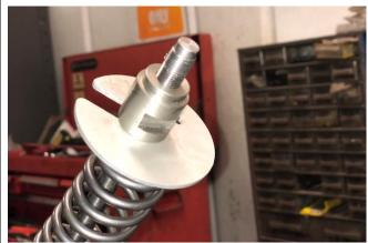
8. Screw on the new preload cap and tighten down by hand until the thread bottoms out, there should be a couple of millimeters gap between the bottom of the preload and the top of the new nut.
