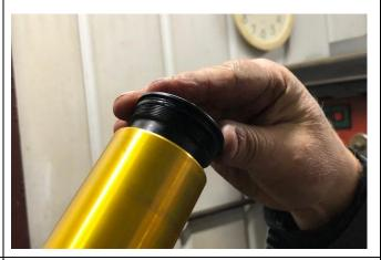
8. Replace the fork leg back into the triple clamp with approximately 10 mm of gold fork tube protruding through the top triple clamp, tighten both lower pinch bolts in bottom triple and then fully tighten the fork cap with the pin spanner provided.
