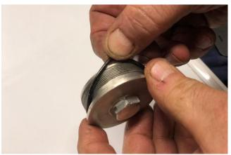
5. Tighten down new fork cap onto damper rod by hand until the thread bottoms out.
