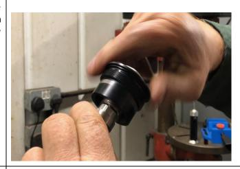
Holding the centre nut of the preload cap with a 22 mm spanner, wind up the new nut on the damper rod with the 16 mm spanner provided and lock the two together.
