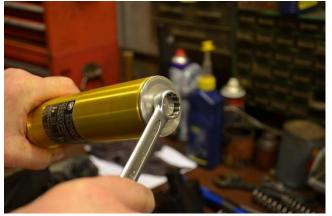
2. Hold lower axle of fork leg in a vice, using soft jaws, and undo fork cap completely.
