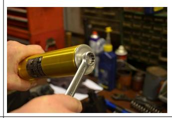
Whilst holding fork cap with 17mm spanner undo the 16 mm locknut underneath on damper rod and remove fork cap, screw locknut back down to bottom of thread by hand.
