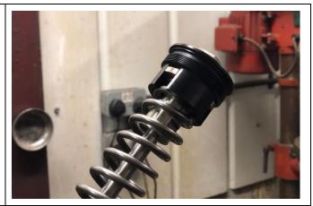
11. Fit the old O ring onto the new preload cap and screw the new preload cap into the outer tube by hand, apply a bit of grease to the O ring before assembly. Hold the gold outer tube by hand and tighten gently the preload cap using the pin spanner provided.
