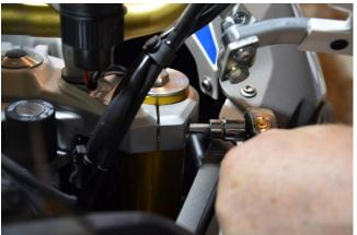
2. Hold lower axle of fork leg in a vice, using soft jaws, and undo fork cap completely with 17mm spanner whilst holding fork tube by hand.
