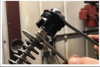
10. Pull down the spring to release the pressure and remove the C washer, then let the spring go back up to seat on the underside of the preload.
