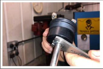
Fit the original O ring onto the new preload cap and screw the new preload cap into the outer tube by hand, apply grease to the O ring before assembly.
