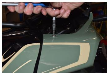
Remove bolts from RH of radiator guard and front fairing
