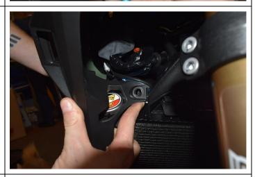
Starting at the bottom, hold the fairing with both hands and ease first out then down to release the spring clip and hook situated inside the fairing panel, this will now leave the fairing free to remove
