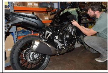
Using a 5mm hex bit undo the top bolt
