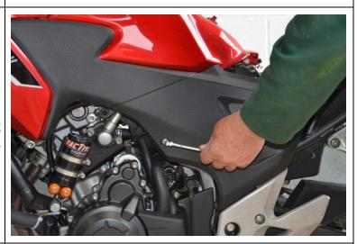
4. Remove both M6 screws and washers from fairing in top of tank, and each stepped M6 screw in side of fairing. Then remove all 4 M6 screws from front of fairing shroud where they connect into front of the radiator.
