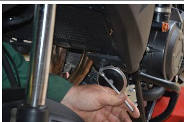
5. Undo both M8 screws and domed nuts that are under front of fairing that attach fairing mount to the headstock. Discard these.
