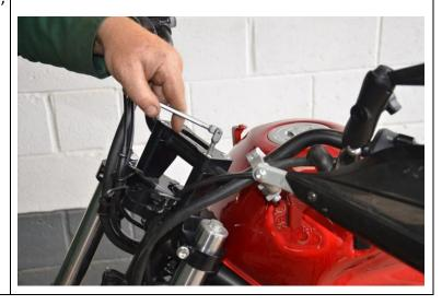
15. Refit both M8 OEM pinch bolts into new triple, using 12mm socket, tighten fully.
