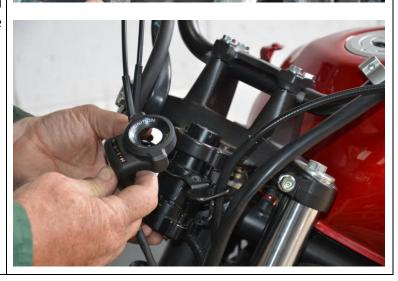
8. Using 9mm drill, remove head of both M8 security screws holding ignition barrel to underside of OEM triple. Pull down ignition barrel and let it hang down.
