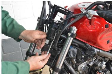
17. Refit plastic ignition cover & wiring guide plate, using both new M5x25 CHS supplied, use Loctite.
