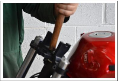
14. Fit bars into top triple & fit top bar clamp, tighten all 4 M8 CHS, but not fully.
