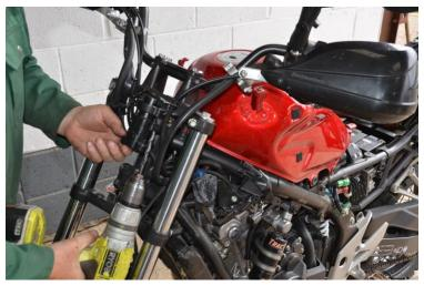
9. Undo all 4 top bar clamp screws with 12mm socket, remove top bar clamp and let bars rotate forward and fall in front of forks.
