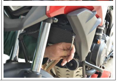
6. Pull fairing forward slightly to expose both wiring connector blocks on left side, disconnect both of these, then gently remove whole fairing assembly.
