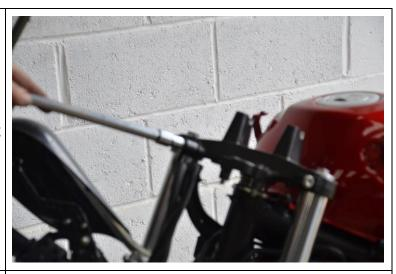
11. If fitting Fork Preload Adjusters RRP 436, or Level 2 or 3 Adventure Kit, undo both OEM fork caps a couple of turns using a 17mm socket. For Level 2 & Level 3 Kit fitting, now is the time to remove the front wheel, front fender and fork legs to change the springs and damper rods.
