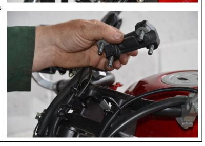
10. Remove both top triple pinch bolts, using 12mm socket, retain these for re-use.
