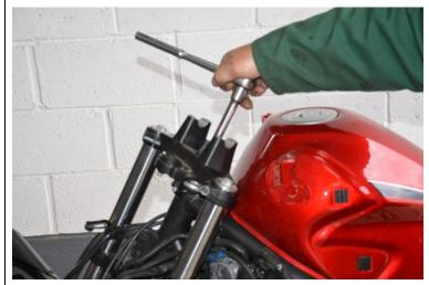
12. Using 30mm socket, undo and remove hex nut and washer holding OEM triple to steering stem, remove top triple. It may need tapping upwards with a soft mallet to remove it.
