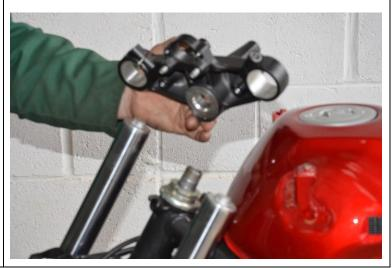
13. Fit new top triple, without top bar clamp, and tap into place with wooden hammer shaft, or similar, to bed down onto headstock. Replace 30mm nut & washer, tighten fully and replace plastic plug.
