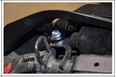
4. Using an 8mm allen key, remove each pillion footrest hanger, then place each Soft Luggage Rack bracket BETWEEN the inside of the footrest hanger and the frame, and ensure the rear of the bracket is BEHIND the bracket on the Soft Luggage rear frames, leave both M10 allen screw footrest bolts loose for now NOTE:It is preferable to use Loctite 248, or
