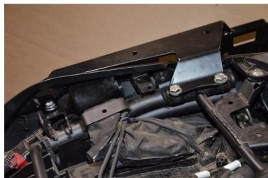
3. Fit 6.5mm thick spacer between underside of front lug and frame, then insert M6x25 screw, and washer, through lug and spacer into frame, do not tighten fully.
