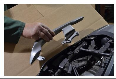
2. Insert front lug on Rear Soft Luggage Rack frame through hole in plastic tail piece, then line up both rear M8 screw holes, and insert both M8x20 screws and washers into each rear hole, do not tighten fully.
