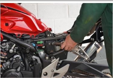
4. Undo the 17mm nuts and remove all 3 of the M10 bolts from triangular linkage plates and discard linkage plates, it is best to mark these before removing, as they are easy to be replaced incorrectly when putting back to standard spec(they are not symmetrical, so be careful).
