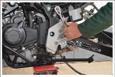
Using a long drift, or screwdriver, push out M10x48mm top bolt, whilst supporting shock body. Gently lower shock out of frame.
