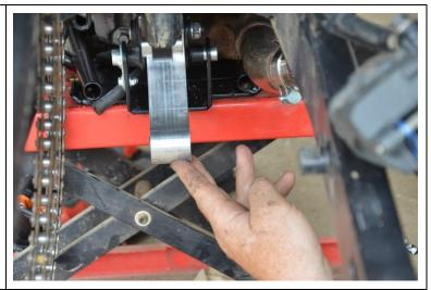
13. Fit both new side plates, LEFT and RIGHT, as marked, insert all 3 M10 bolts, tighten all 3 M10 nuts(no washers) to 40Nm. It may be necessary to "jiggle" the swinging arm up and down slightly to get all 3 screws in position.
