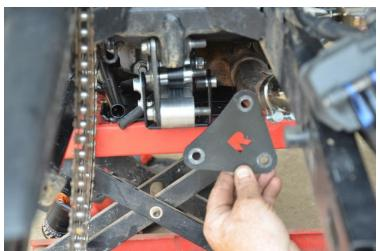
14. Replace rectifier, use Loctite, or similar, on both M6 screws.
