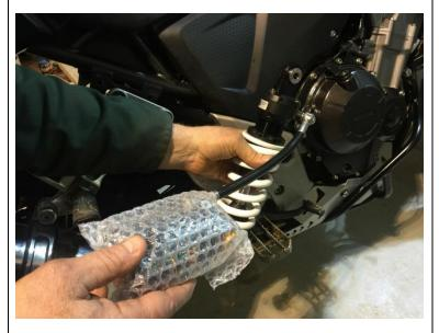
9. The shock reservoir needs to be fed through the right side, below the frame and behind the footrest hanger. It needs to pass above the rear brake hose that is attached to the swinging arm and in front of the low pressure hose that feeds the master cylinder.
