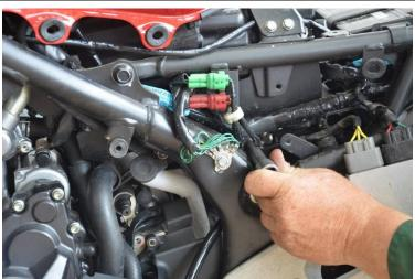
11. Remove both M8 screws holding right hand passenger footrest hanger, using 8mm Allen key. Slide in new reservoir mount between footrest hanger and frame and re-insert both M8 screws. (using Loctite or similar) Tighten to 26Nm.
