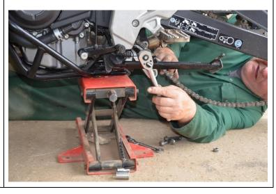
6. Remove top shock bolt nut by holding the bolt(from left side) securely with an 8mm Allen key, then undo the 17mm nut and remove both nut and washer from the right side. It is best to use a 3/8" drive deep 17mm socket and extension bar through the rubber flap between the starter solenoid and frame. DO NOT LOSE WASHER.
