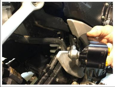
10. Insert top shock bolt, M10x48mm, from left side, through frame and top shock mount. Replace washer and M10 nut on right side, tighten to 40Nm.
