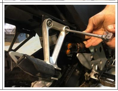
12. Fit new lower link and insert front M10x58mm bolt, tighten M10 nut (no washer) to 40Nm, using 8mm Allen key and 17mm socket.
