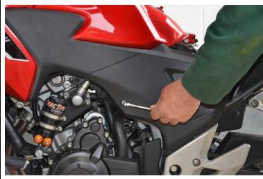
3. Remove both M6 screws securing rectifier to frame, using a 10mm socket, and let rectifier hang down, in order to access top shock bolt.
