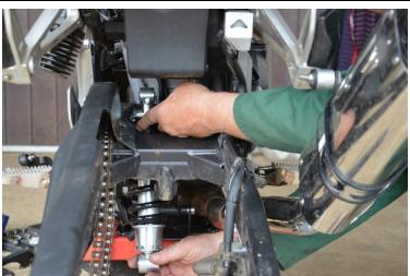
Insert new shock up through gap between swinging arm brace and rear of engine, with the shock positioned as shown, with the hose outlet at the 2 'O' Clock position (when viewed from rear of bike facing forward)
