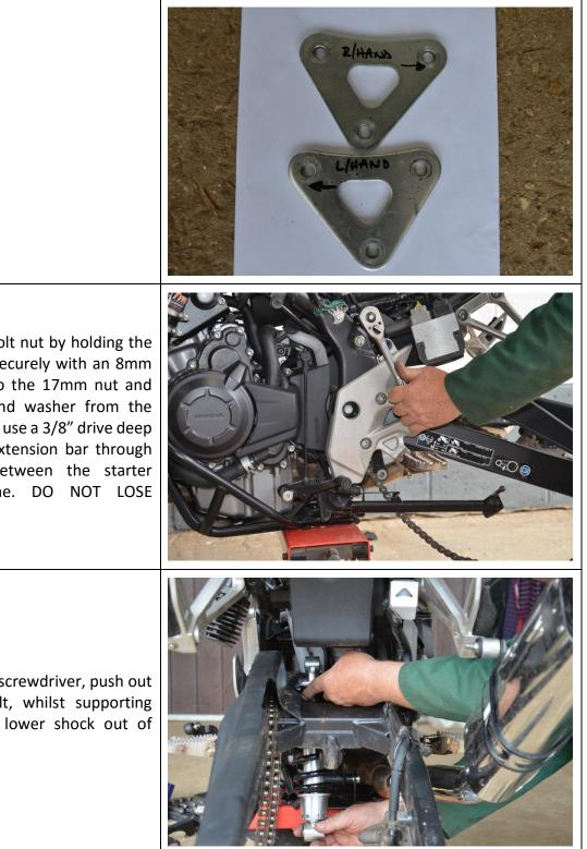
5. Remove top shock bolt nut by holding the bolt(from left side) securely with an 8mm Allen key, then undo the 17mm nut and remove both nut and washer from the right side. It is best to use a 3/8" drive deep 17mm socket and extension bar through the rubber flap between the starter solenoid and frame. DO NOT LOSE WASHER.
