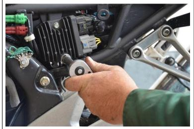
10. Replace rectifier, use Loctite, or similar, on both M6 screws.
