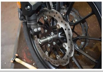
31. Slide axle through the right-hand fork leg, and through the front wheel. The when the axle is fully inserted secure with bolt from opposite side, tighten fully using 14mm hex bit on right axle end and 19mm spanner on left end.
