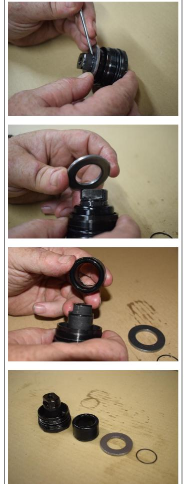
14. Take the new Rally Raid fork cap, insert the rubber sleeve, then the metal washer and finally the wire clip, making sure the clip is seated in the groove.
