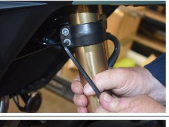
Using a 45mm spanner, undo the right-hand fork cap about one turn. Whilst holding the lower fork leg undo both lower triple pinch bolts and remove whole leg.
