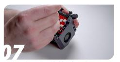
Unscrew the M3 BHCS holding the probe using a 2 mm hex key.
