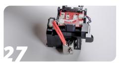
Add the thermistor and the heater cartridge to the hotend.
