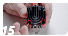
Take your LGX ACE and unscrew the two screws holding the hotend to the extruder from the front using a 2 mm hex key.
