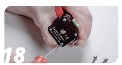
Unscrew the top right and bottom left screws on the extruder motor as seen from the back using a Philips head screwdriver.
