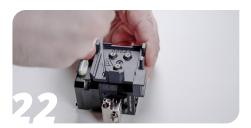
Add the assembly to the ACE and tighten the screws using a 2 mm hex key.
